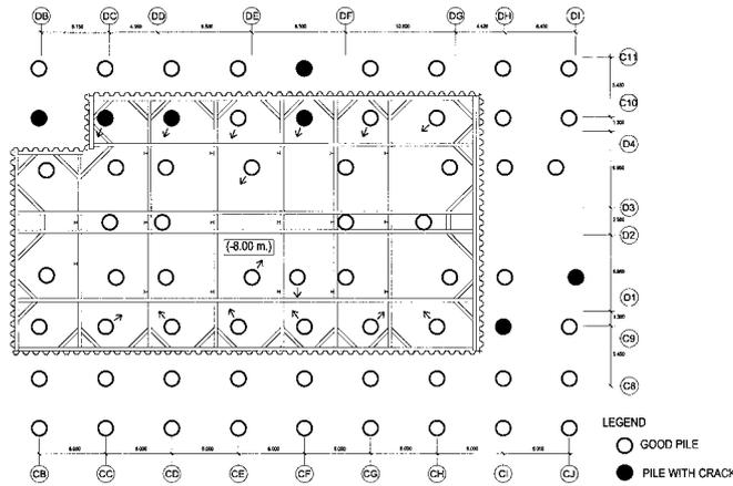
Figure 3. Plan of Excavation and Location of Damaged Piles and Pile Movements (a Portion of Project Area) Case III
