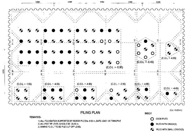
Figure 4. Plan of Excavation and Location of Damaged Piles (a Portion of Project Area) Case IV
