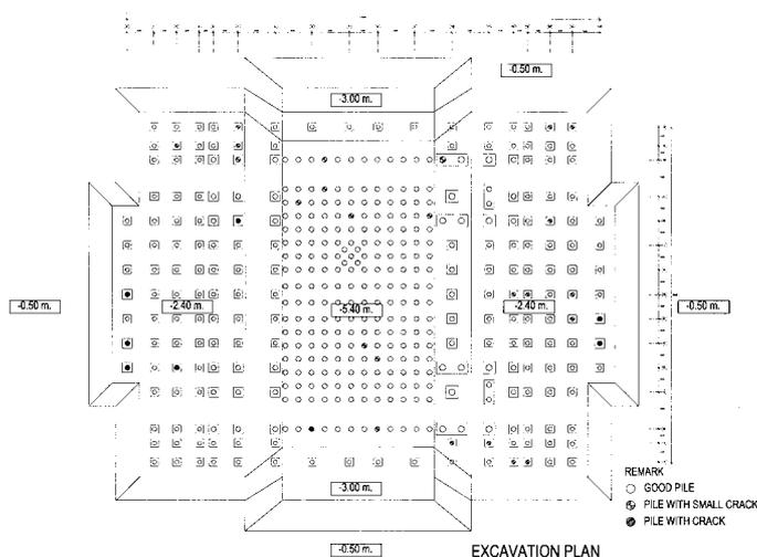
Figure 1. Excavation Plan and Location of Damaged Piles
