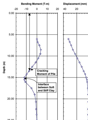
Figure 10. Computed Bending Moment in Pile and Pile's Deflection Closest to Sheet Pile Wall - Case IV
