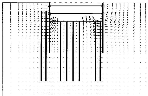
Figure 11. Section Showing Displacements of Soil - Case IV
