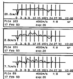
Figure 5. Sonic Integrity Test Records showing Good pile, Pile with less Prominent Crack and Prominent Crack respectively - Case IV.
