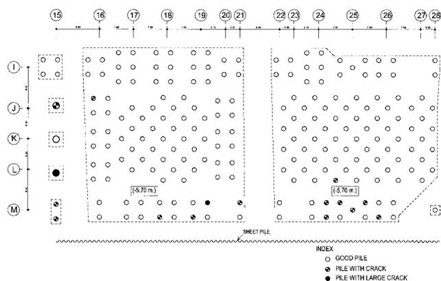
Figure 2. Location of Damaged Piles (only a quarter of Project Site shown here) Case II
