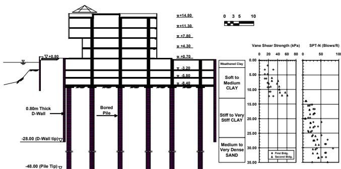
Figure 2. Basement section and soil profile (Second Building)
