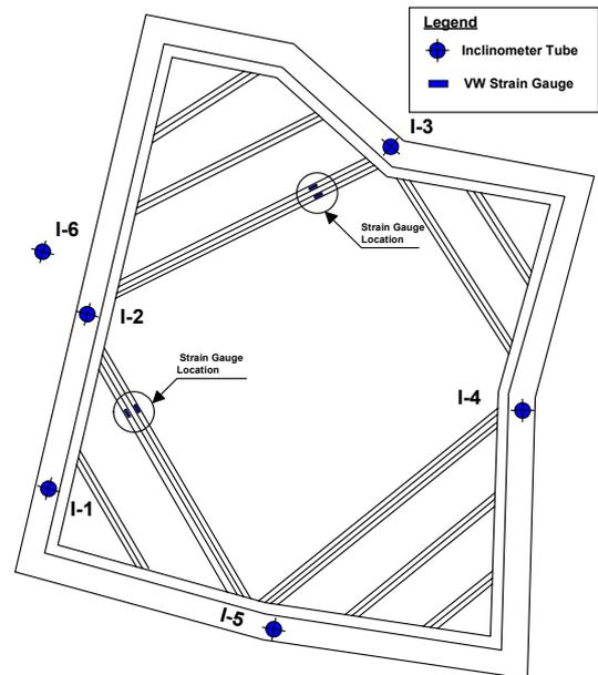
Figure 11. Arrangement of strutting system with stain gauges (after EIT 1999)
