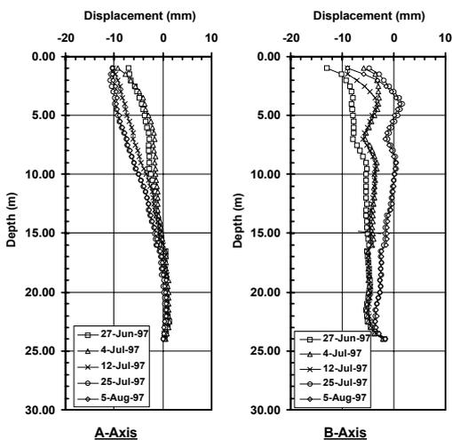
Figure 4b. Inclinometer reading of I-4
