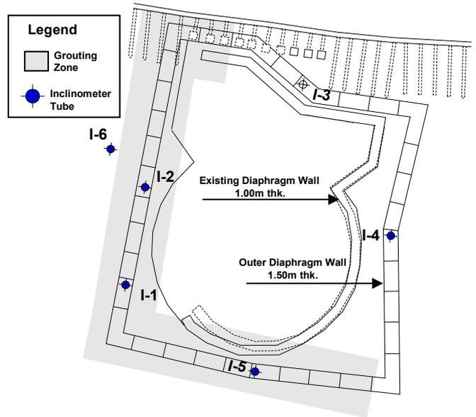
Figure 10. Location of inclinometers and treated area by Jet grouting (after EIT 1999)
