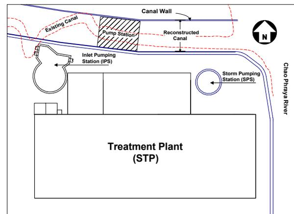
Figure 1. Layout of Inlet Pumping Station
