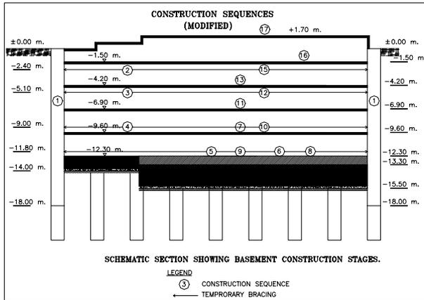
Fig. 4 The Modified Construction Sequence
