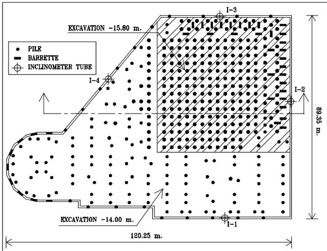
Fig. 2 Layout Plan of Diaphragm Wall & Piles
