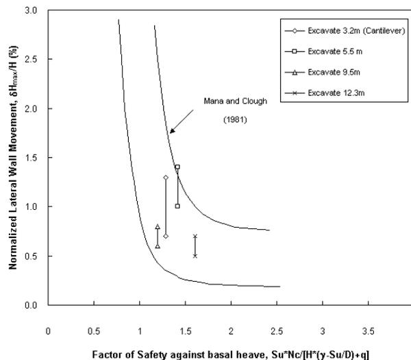
Fig. 10 Relationship between Normalized Maximum lateral movement versus factor of safety against basal heave.
