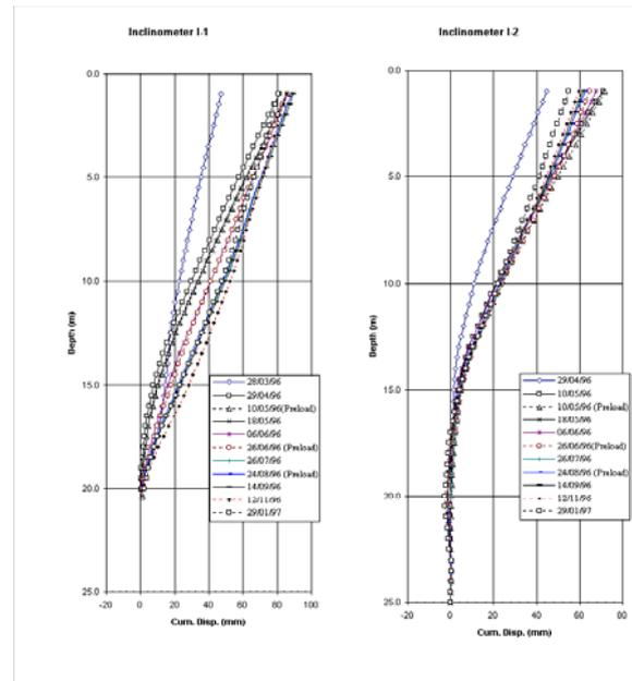
Fig. 6A. Lateral Movements of the wall shown by Inclinometer Tubes I-1 and I-2.
