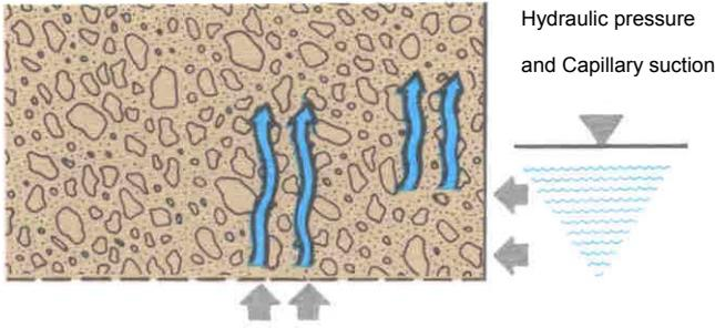
Figure 4. Capillary suction and hydraulic pressure in concrete
