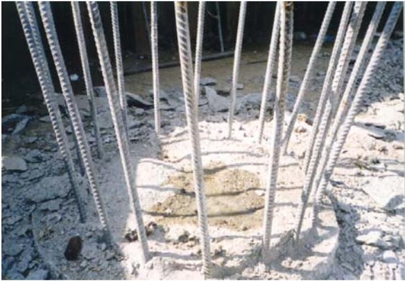
Figure 5. Wet pile head caused by capillary flow of ground water through segregated concrete in the pile
