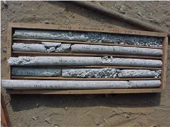
Figure 6. Core samples showing segregated concrete in the pile
