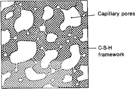
Figure 2. Low permeability of concrete caused by less interconnecting voids
