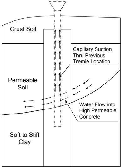
Figure 3. Capillary flow of ground water in bored pile
