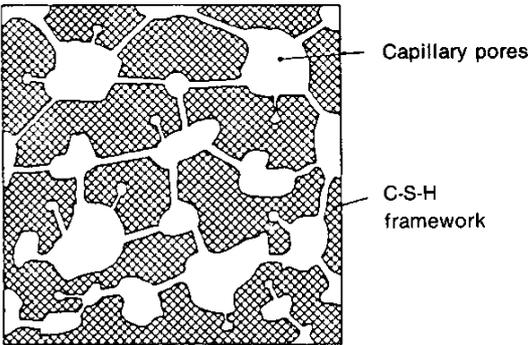
Figure 1. High permeability of concrete caused by interconnecting voids
