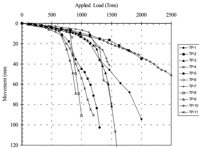
Figure 3. Load settlement curves of the test piles.
