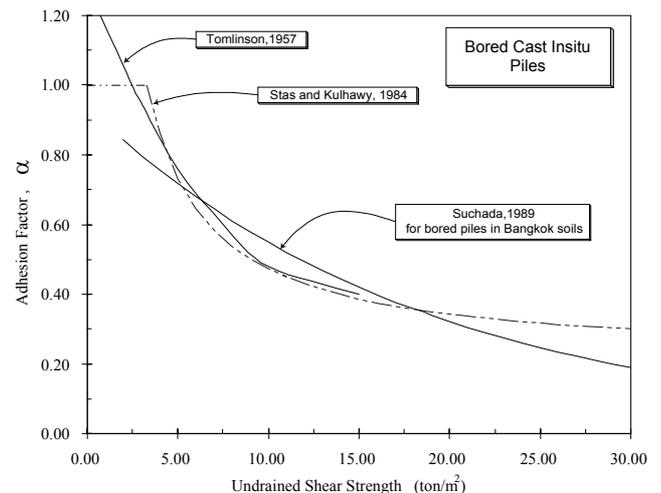
Figure 2. Comparison of Adhesion factor  $\alpha$  used for bored piles in Bangkok Subsoils.
