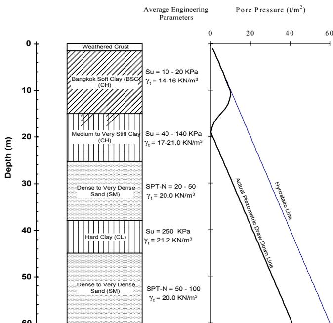
Figure 1. Typical soil profile of Bangkok plain with piezometric draw down conditions.
