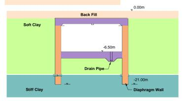
Schematic section of cut and cover tunnel.
